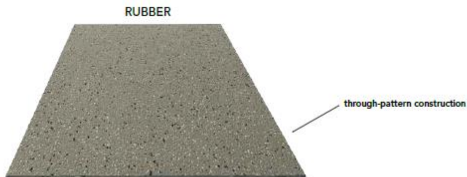
Figure 1: Diagram of Rubber Floor Tile Cross-Section
